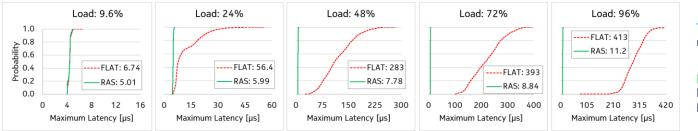
Test: uniform traffic from *identical* flows, multiple load levels
