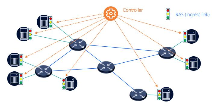
The RAS and the controller can be implemented as software modules and deployed on demand, as a service
